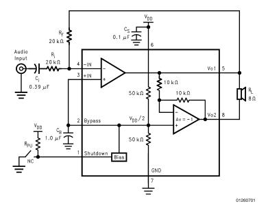
FIGURE 1. Typical Audio Amplifier Application Circuit
