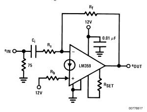
Determine the required I<sub>SET</sub> from the characteristic curves for gain bandwidth product.
