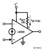
$$I_{SET(IN)} = \frac{V^+ - V_{BE}}{R_{SET(IN)} + 500\Omega}$$
