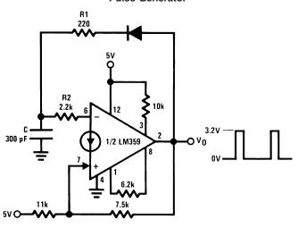
Output is TTL compatible Duty cycle is adjusted by R1 Frequency is adjusted by C f = 1 MHz Duty cycle = 20%
