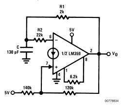
f=1 MHz Output is TTL compatible Frequency is adjusted by R1 & C (R1  $\, \, \stackrel{<}{<} \, \, \, \text{R2})$
