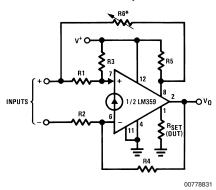
$$V_{O(DC)} = \frac{R4}{R3}(V^+ - \varphi) \mbox{ where } \varphi = 0.6V$$
