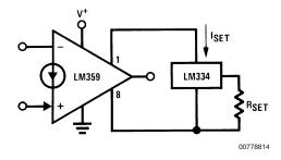
$$I_{SET} = \frac{67.7 \text{ mV}}{R_{SET}} @25^{\circ}\text{C}$$
