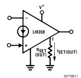
$I_{SET(OUT)} = \frac{V^{+} - V_{BE}}{R_{SET(OUT)} + 500\Omega}$
