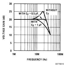
$$\begin{split} &V_{o(DC)} = 5.1V\\ &\text{Differential phase error} \le 1^{\circ} \text{ for } 3.58 \text{ MHz } f_{IN}\\ &\text{Differential gain error} \le 0.5\% \text{ for } 3.58 \text{ MHz } f_{IN}\\ &f_{-3 \text{ dB}} \text{ low} = 2.5 \text{ Hz} \end{split}$$
