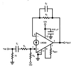
2. Select I<sub>SET</sub> to provide adequate amplifier bandwidth so that the closed loop bandwidth will be determined by R<sub>f</sub> and C<sub>f</sub>. To do this, the set current should program an amplifier open loop gain of at least 20 dB at the desired closed loop bandwidth of the circuit. For this example, an I<sub>SET</sub> of 0.5 mA will provide 26 dB of open loop gain at 20 MHz which will be sufficient. Using single resistor programming for I<sub>SET</sub>:
