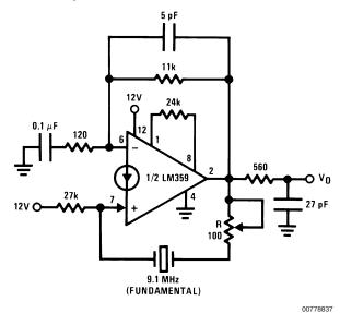
$V_0 = 500 \text{ mVp-p}$  f = 9.1 MHz $THD \le 2.5\%$
