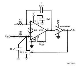
$$\begin{split} f_0 &= \frac{V_{IN} - \varphi}{4 \, C \Delta V \, R1} \\ \text{where: } R2 &= \, 2R1 \\ &\varphi = \text{amplifier input voltage} \, = \, 0.6V \\ &\Delta V = \, DM7414 \, \text{hysteresis, typ 1V} \end{split}$$
