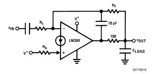
FIGURE 11. Isolating Large Capacitive Loads
