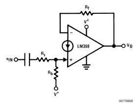
$$\begin{split} A_{V(AC)} &= \, + \frac{R_f}{R_s + r_e} \\ V_{o(DC)} &= V_{BE}(-) + \, R_f \left[ \frac{V^+ - V_{BE}(+)}{R_b} + I_b(-) \right] \end{split}$$
