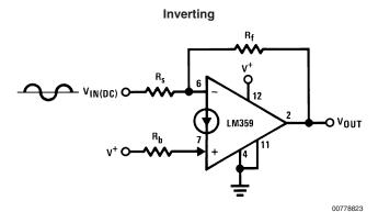
$$\begin{split} V_{O(DC)} &= \left[\frac{V^+ - V_{BE}(+)}{R_b} - \frac{V_{IN(DC)} - V_{BE}(-)}{R_s}\right] R_f + V_{BE}(-) \\ A_{V(AC)} &= \frac{R_f}{R_s} \end{split}$$
