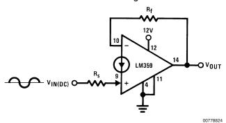
$$\begin{split} V_{o(DC)} &= V_{BE}(-) \, + \, \frac{(V_{IN(DC)} - V_{BE}(+)) \, R_f}{R_s} \\ A_{V(AC)} &= \, + \frac{R_f}{R_s \, + r_e(+)} \end{split}$$
