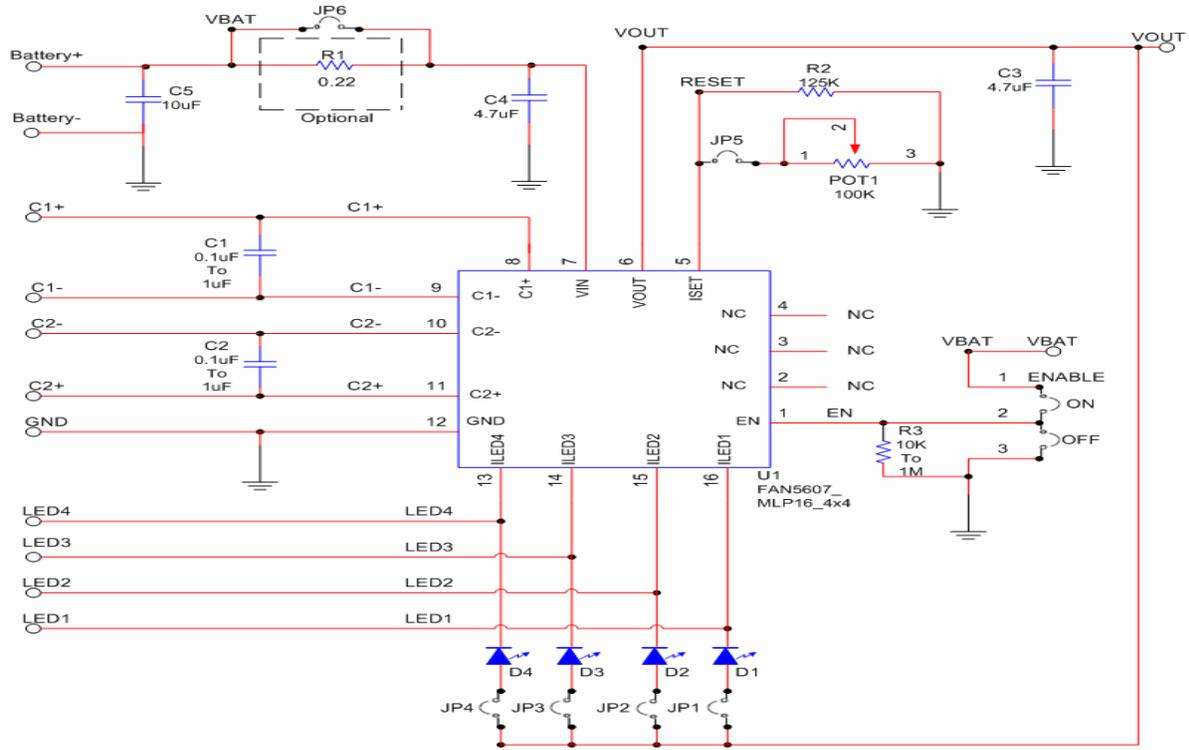
Figure 2: Schematic Diagram
