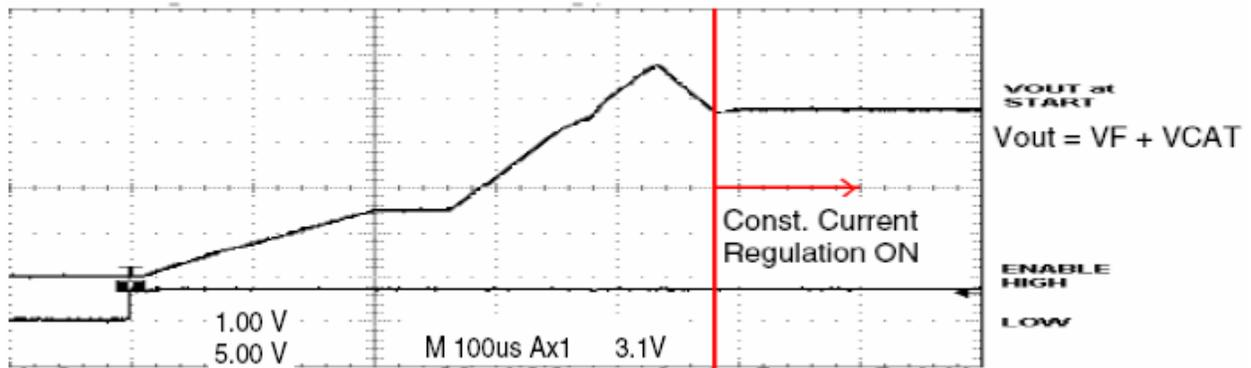
Figure 4: Start-Up Waveform
