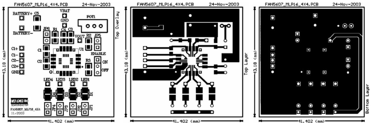
Figure 3: PCB Layout
