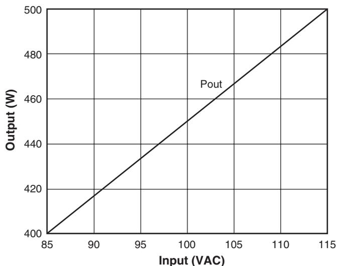
**Figure 1. Output Power vs. Line Voltage**
