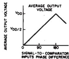
Fig. 4—Phase-comparator I characteristics at low-pass filter output.
