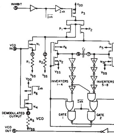
Fig. 8 - Schematic of COS/MOS VCO section.
