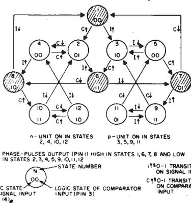
Fig. 7 - State diagram of phase-comparator II.
