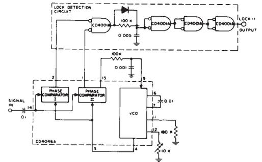
Fig. 15— Lock-detection circuit.
