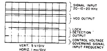
Fig. 16— Lock-detection-circuit waveforms.
