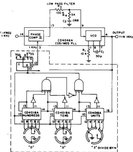
Fig. 12— Low-frequency synthesizer with three-decade programmable divider.
