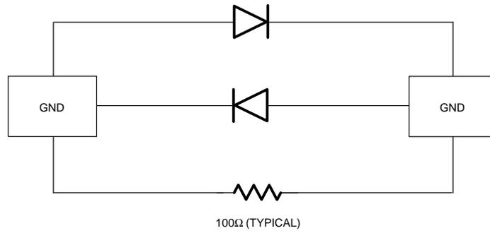
**NOTE:** GND and AGND must be tied to the same voltage level.
