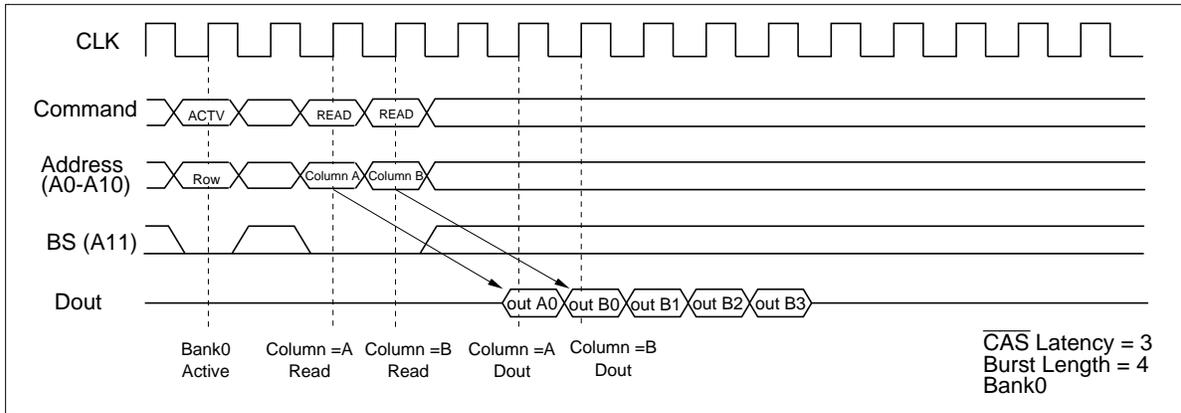
**Same bank, different ROW address:** When the ROW address changes on same bank, consecutive read commands cannot be executed; it is necessary to separate the two read commands with a precharge command and a bank-active command.
