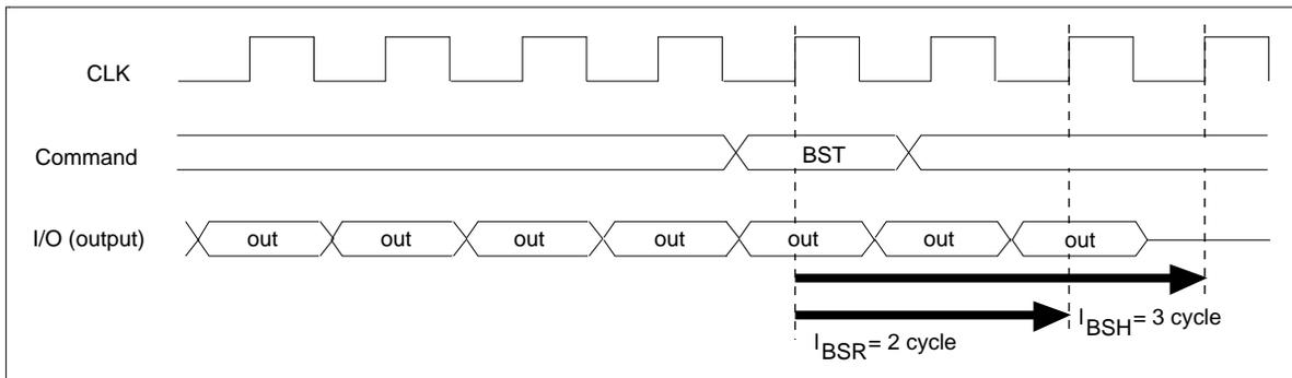
**Burst stop command at burst write:** The burst stop command (BST command) is used to stop data input during a full-page burst write. No data is written in the same cycle as the BST command and in subsequent cycles. In addition, the BST command is only valid during full-page burst mode, and is invalid with burst lengths of 1, 2, 4 and 8. And an interval of  $t_{DPL}$  is required between the BST command and the next precharge command.
