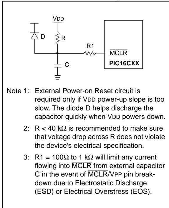
**FIGURE 8-13: EXTERNAL BROWN-OUT PROTECTION CIRCUIT 1**
