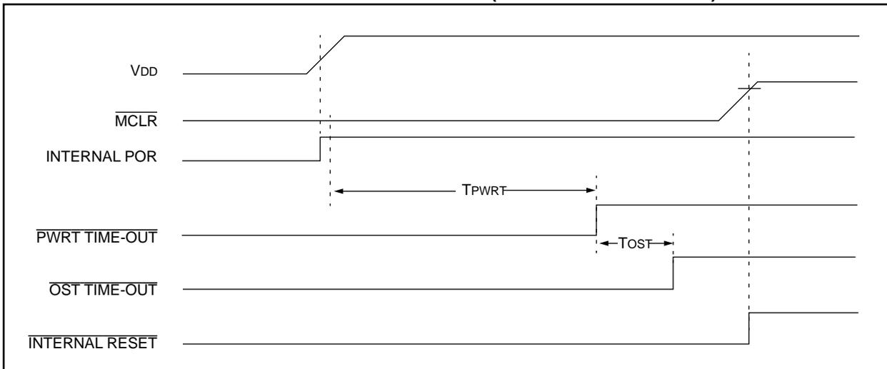
**FIGURE 8-11: TIME-OUT SEQUENCE ON POWER-UP ( $\overline{\text{MCLR}}$  TIED TO  $V_{\text{DD}}$ )**
