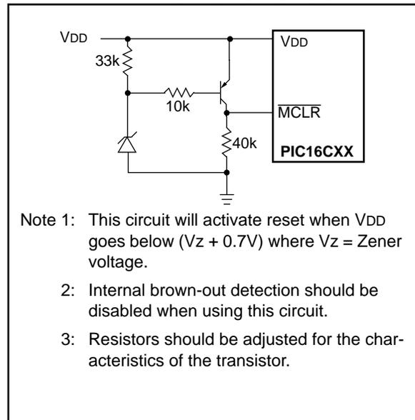
**FIGURE 8-14: EXTERNAL BROWN-OUT PROTECTION CIRCUIT 2**
