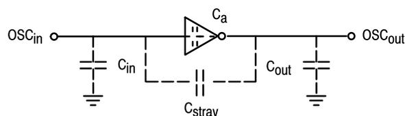
Figure 19. Parasitic Capacitances of the Amplifier and C<sub>stray</sub>
