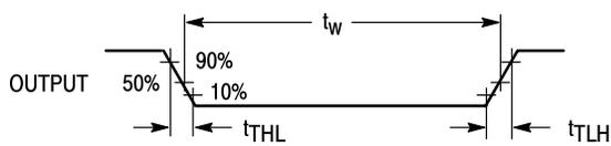
Figure 11. Switching Waveform
