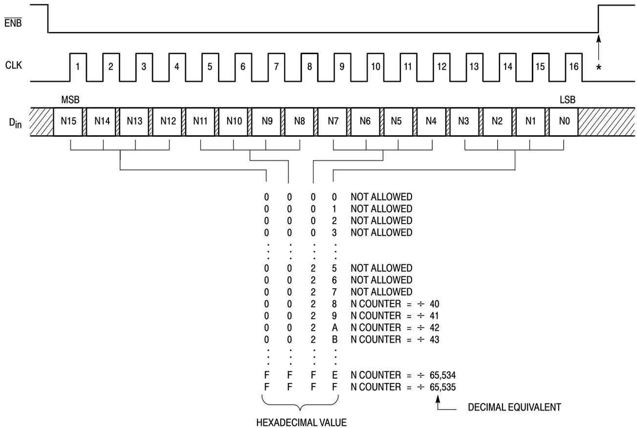
\* At this point, the two new bytes are transferred to the N register and stored. No other registers are affected. In addition, the N and R counters are jam-loaded and begin counting down together.
