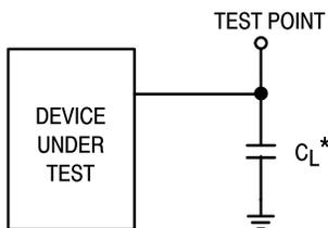
\* Includes all probe and fixture capacitance.
