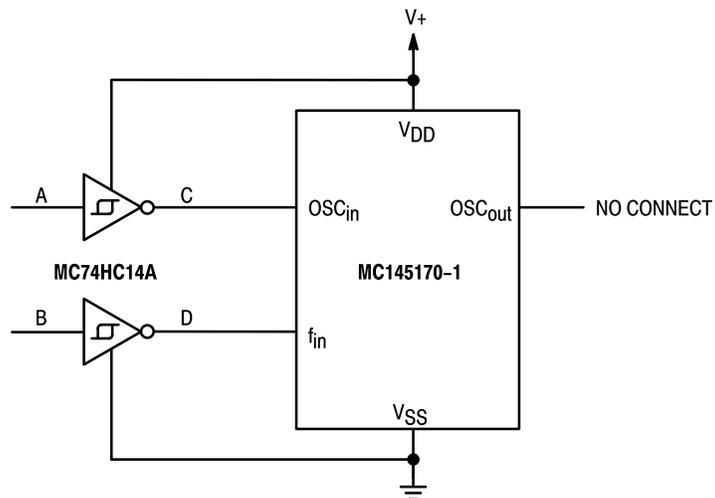
NOTE: The signals at Points A and B may be low-frequency sinusoidal or square waves with slow edge rates or noisy signal edges. At Points C and D, the signals are cleaned up, have sharp edge rates, and rail-to-rail signal swings. With signals as described at Points C and D, the MC145170-1 is guaranteed to operate down to a frequency as low as dc.
