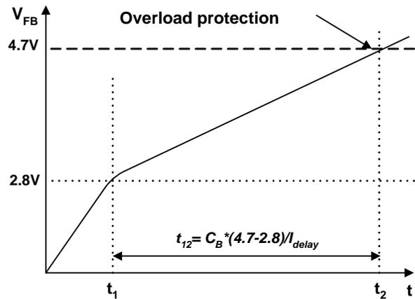
**Figure 17. Overload Protection**
