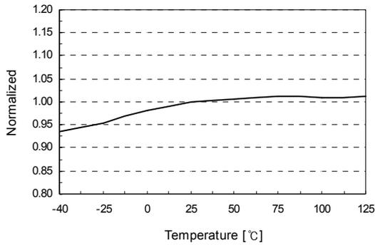
**Figure 10. Feedback Source Current (I<sub>FB</sub>) vs. T<sub>A</sub>**
