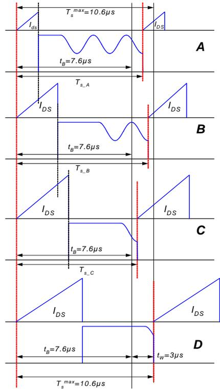
**Figure 19. Advanced VS Operation**
