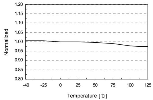
Figure 5. Peak Current Limit ( $I_{\text{LIM}}$ ) vs.  $T_A$
