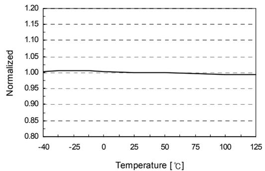
Figure 9. Maximum Duty Cycle ( $D_{\text{MAX}}$ ) vs.  $T_A$
