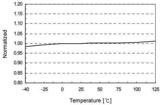
**Figure 12. Operating Supply Current (I<sub>OP</sub>) vs. T<sub>A</sub>**
