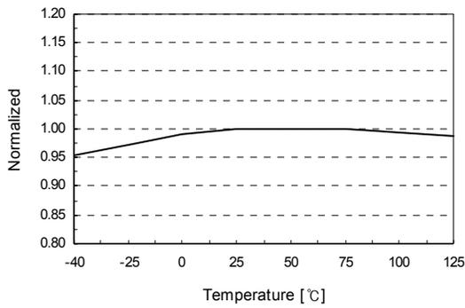
Figure 4. Operating Frequency ( $f_{\text{OSC}}$ ) vs.  $T_A$
