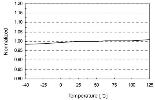
Figure 7. Stop Threshold Voltage ( $V_{\text{STOP}}$ ) vs.  $T_A$
