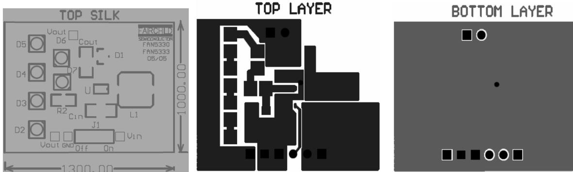
Figure 3: PCB Layout
