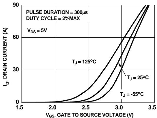
Figure 5. Transfer Characteristics
