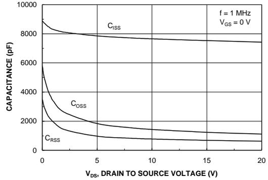
Figure 8. Capacitance Characteristics.
