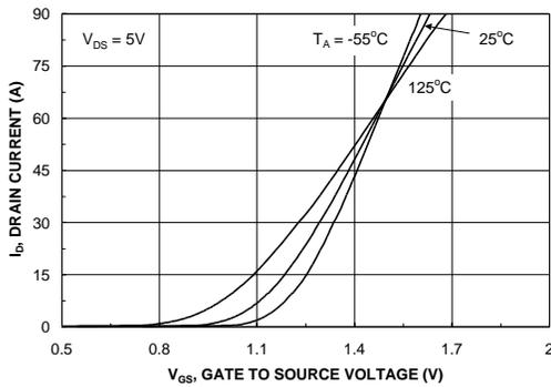
Figure 5. Transfer Characteristics.
