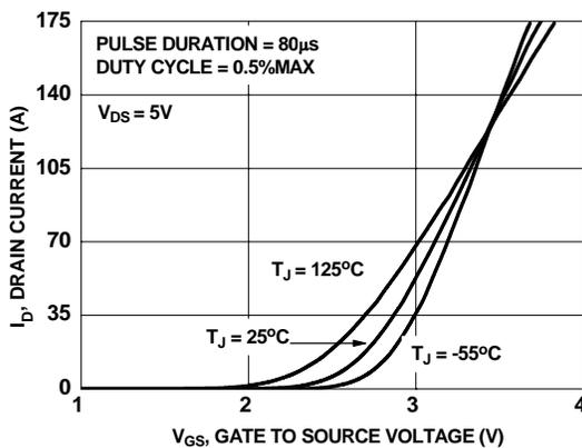
Figure 5. Transfer Characteristics
