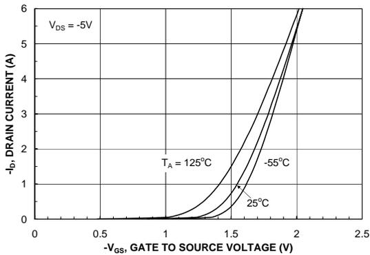
Figure 5. Transfer Characteristics.
