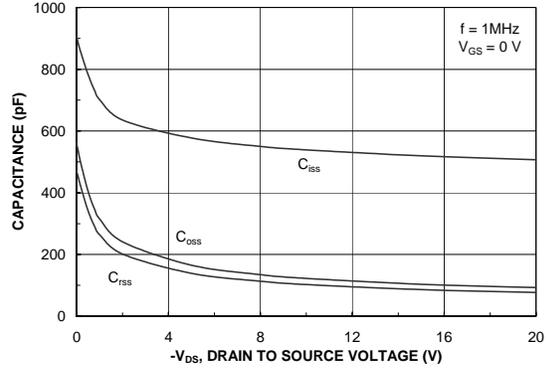
Figure 8. Capacitance Characteristics.
