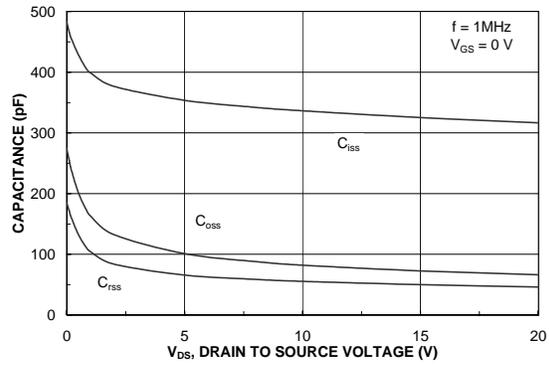
Figure 8. Capacitance Characteristics.
