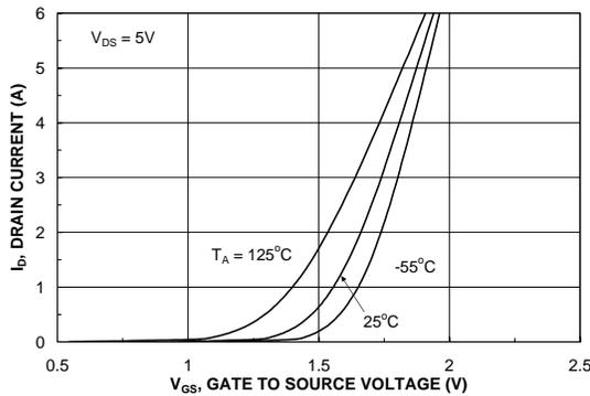
Figure 5. Transfer Characteristics.
