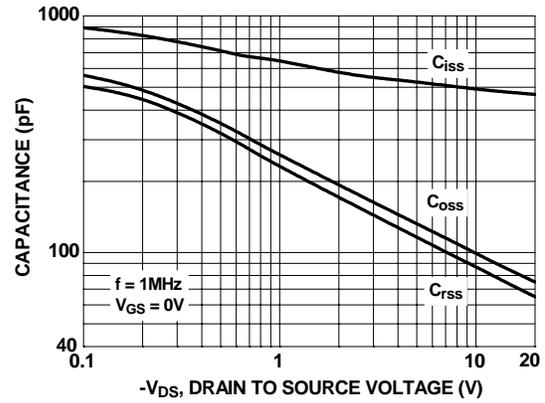
**Figure 8. Capacitance Characteristics**
