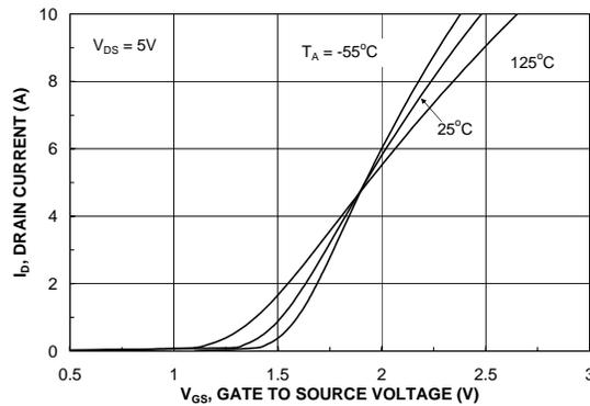
Figure 5. Transfer Characteristics.
