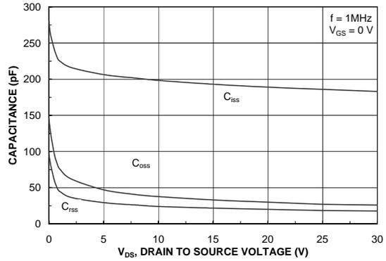
Figure 8. Capacitance Characteristics.
