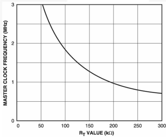
Figure 4. Master Clock Frequency vs. R<sub>T</sub>
