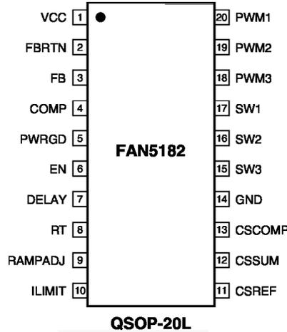
Figure 2. Pin Assignments
