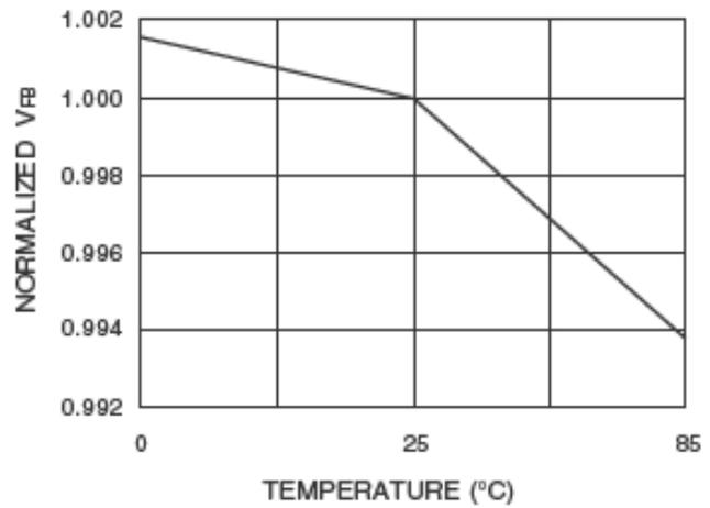
Figure 5. Normalized V<sub>FB</sub> vs. Temperature
