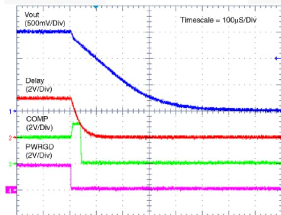
Figure 10. Shutdown Waveforms
