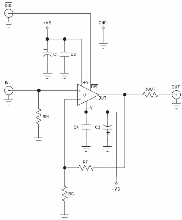
Figure 26. FAN4174 Evaluation Board Schematic (KEV002/KEB011)
