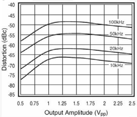
Figure 16. 3rd Harmonic Distortion vs.  $V_O$
