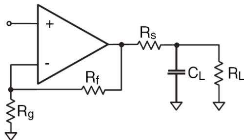
Figure 25. Typical Topology for Driving a Capacitive Load
