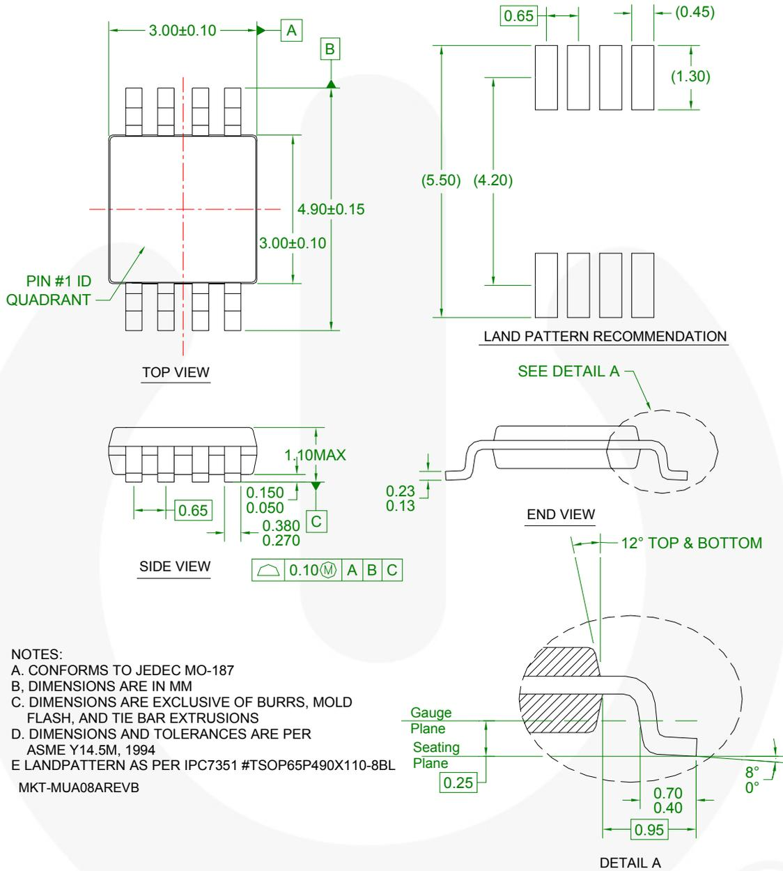
**Figure 34. 8-Lead Molded Small Outline (MSOP) Package**
