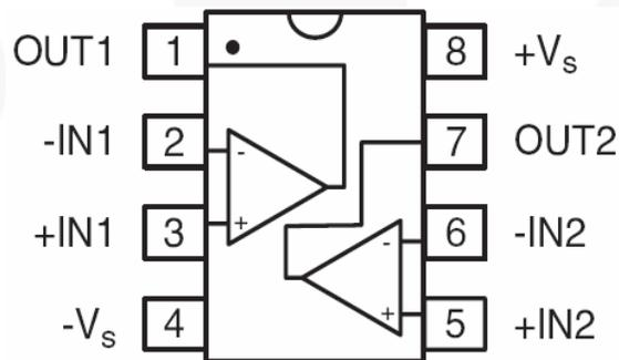
Figure 5. FAN4274 MSOP
