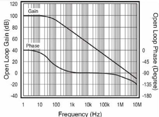
Figure 13. Open-loop Gain and Phase vs. Frequency
