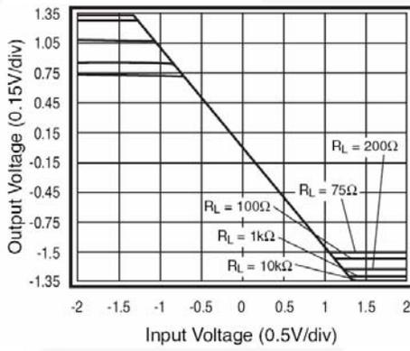
Figure 19. Output Swing vs. Load
