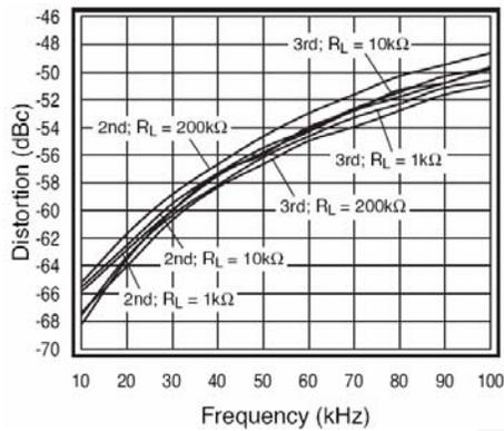
Figure 14. 2nd and 3rd Harmonic Distortion
