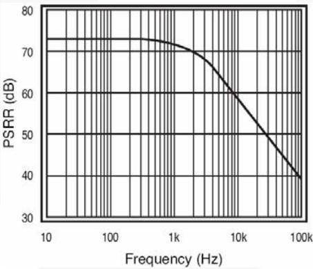
Figure 18. PSRR  $V_S=5V$
