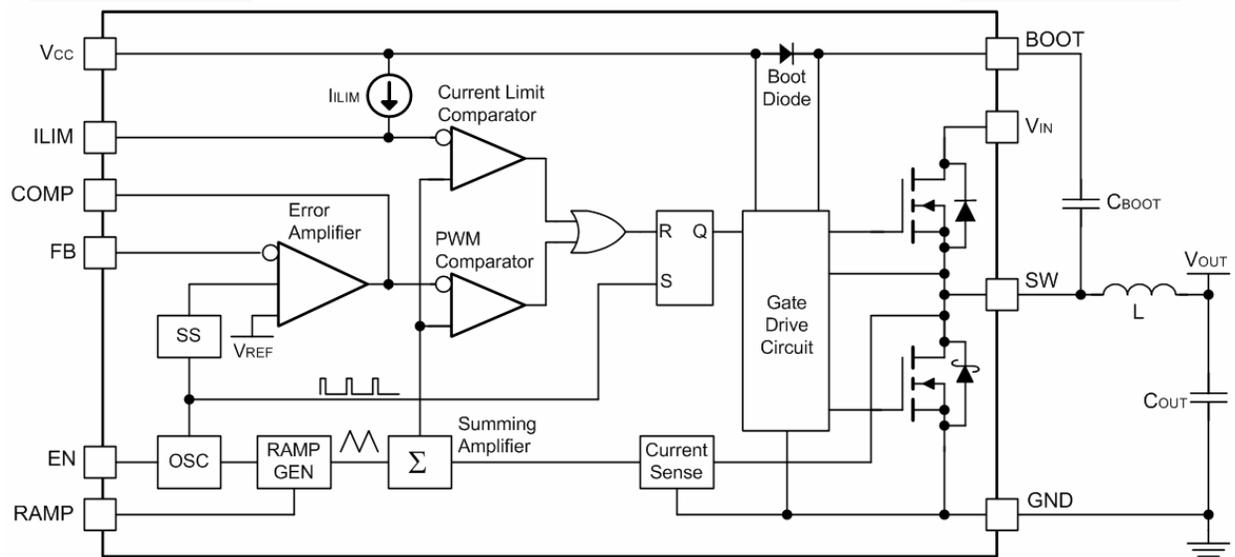
Figure 2. Block Diagram
