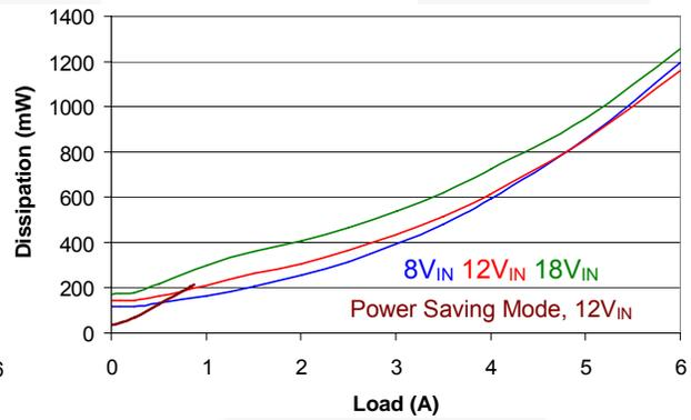
Figure 12. 1.8V<sub>OUT</sub> Dissipation Over V<sub>IN</sub> vs. Load
