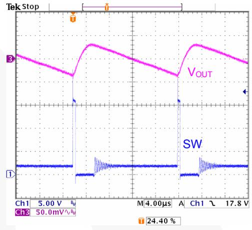
Figure 16. SW and  $V_{OUT}$  Ripple, 0.3A Load
