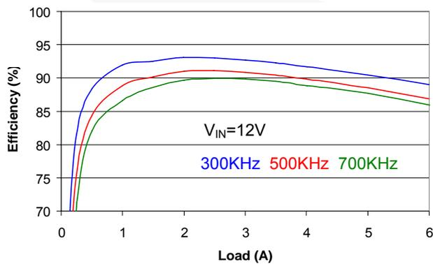
Figure 13. 1.8V<sub>OUT</sub> Efficiency Over Frequency vs. Load (Circuit Value Changes)
