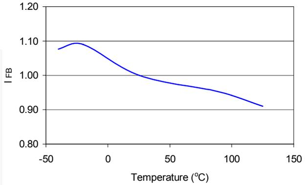
**Figure 5. Reference Bias Current ( $I_{FB}$ ) vs. Temperature, Normalized**
