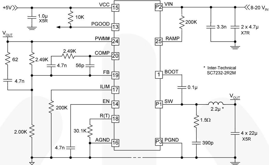
Figure 10. Application Circuit: 1.8V<sub>OUT</sub>, 500KHz
