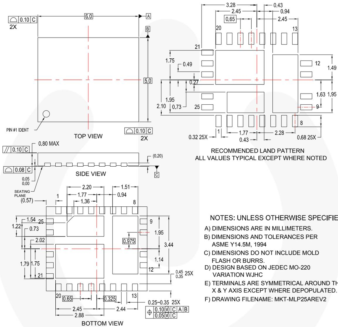
**Figure 27. 5x6mm Molded Leadless Package (MLP)**
