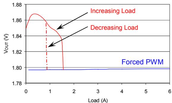
**Figure 25. Power-Saving Mode Regulation (Using Figure 10 Circuit)**
