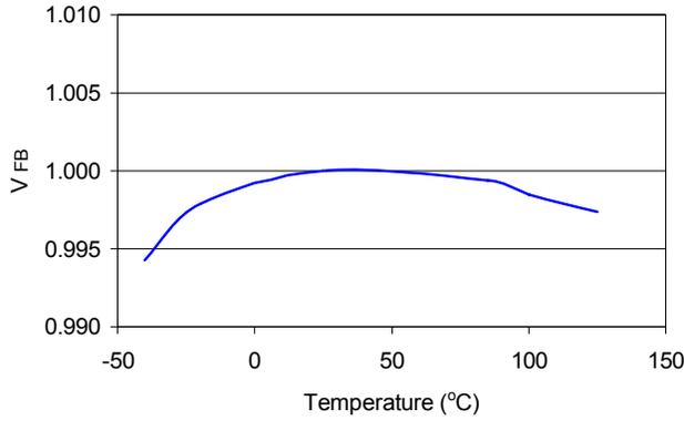
**Figure 4. Reference Voltage ( $V_{FB}$ ) vs. Temperature, Normalized**
