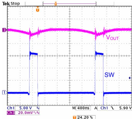
Figure 15. SW and  $V_{OUT}$  Ripple, 6A Load
