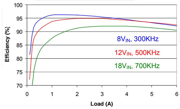
Figure 14. 3.3V<sub>OUT</sub> Efficiency vs. Load (Circuit Value Changes)
