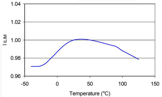
**Figure 9.  $I_{ILIM}$  Current ( $I_{ILIM}$ ) vs. Temperature, Normalized**
