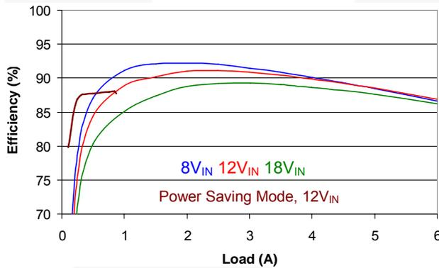
Figure 11. 1.8V<sub>OUT</sub> Efficiency Over V<sub>IN</sub> vs. Load
