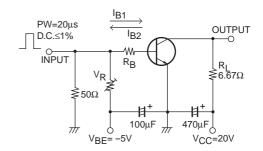
$20I_{B1} = -20I_{B2} = I_C = 3A$ For PNP, the polarity is reversed.
