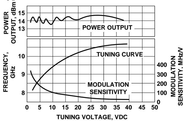
Figure 13. VTO-8850 Power Output, Frequency and Modulation Sensitivity vs. Tuning Voltage.
