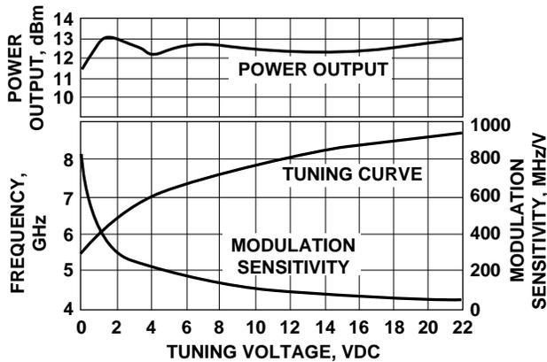
Figure 11. VTO-8650 Power Output, Frequency and Modulation Sensitivity vs. Tuning Voltage.
