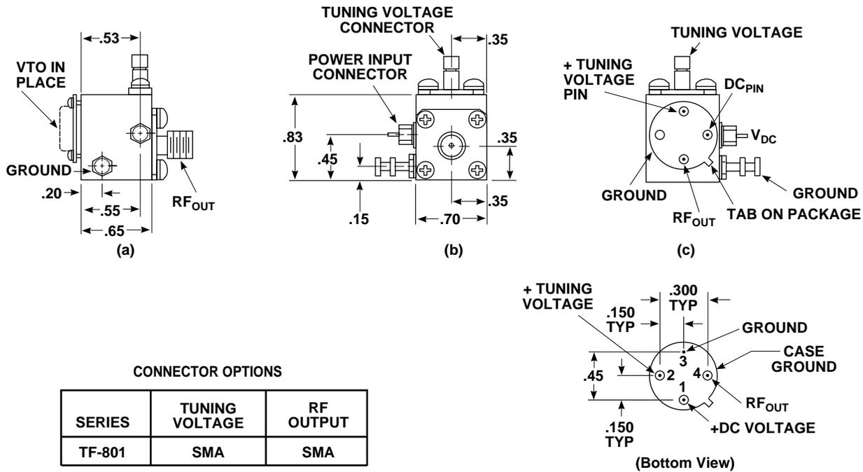
Figure 15. TO-8 Test Fixture.
