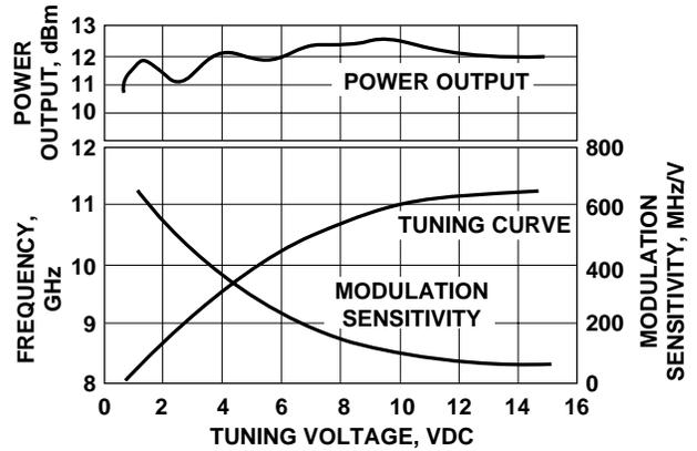
Figure 14. VTO-8950 Power Output, Frequency and Modulation Sensitivity vs. Tuning Voltage.
