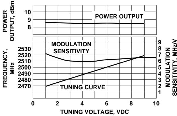
Figure 7. VTO-8248 Power Output, Frequency and Modulation Sensitivity vs. Tuning Voltage.
