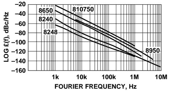
Figure 16. Noise Comparison Single Sideband Phase Noise.
