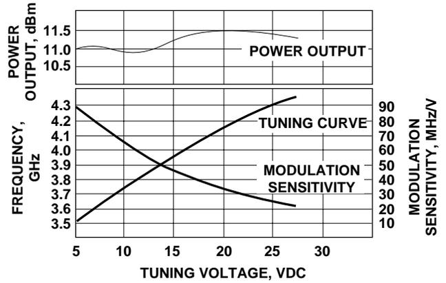
Figure 8. VTO-8360 Power Output, Frequency and Modulation Sensitivity vs. Tuning Voltage.
