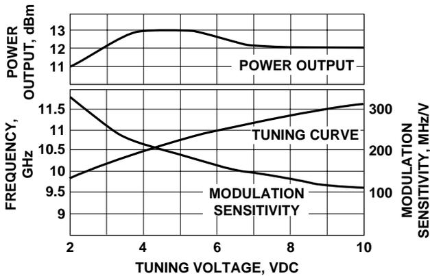
Figure 15. VTO-810750 Power Output, Frequency and Modulation Sensitivity vs. Tuning Voltage.
