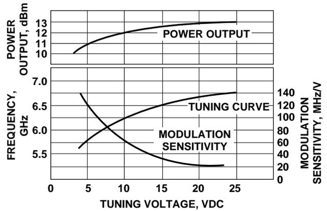
Figure 10. VTO-8580 Power Output, Frequency and Modulation Sensitivity vs. Tuning Voltage.
