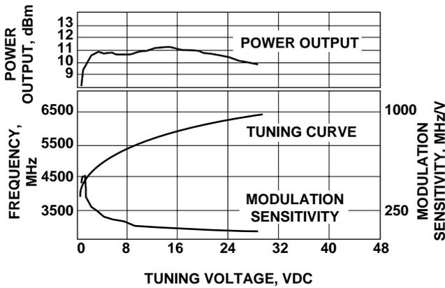
Figure 9. VTO-8430 Power Output, Frequency and Modulation Sensitivity vs. Tuning Voltage.
