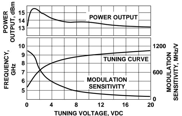
Figure 12. VTO-8810 Power Output, Frequency and Modulation Sensitivity vs. Tuning Voltage.
