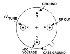
necessary RF filtering action yet as low as possible to maximize  $\Delta V/\Delta T$  characteristics for excellent tuning speeds. Used in a phase locked loop PLL circuit, a VTO provides a receiver LO with stability equivalent to the reference oscillator (usually crystal controlled), yet variable in discrete steps or continuously depending on the PLL configuration.
