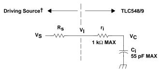
V<sub>I</sub> = Input Voltage at ANALOG IN
