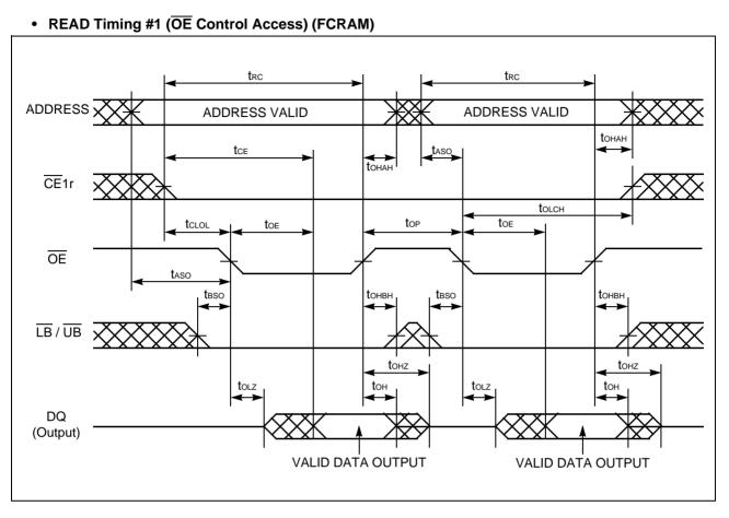
Note: CE2r,  $\overrightarrow{PE}$  and  $\overrightarrow{WE}$  must be High for entire read cycle. Either or both LB and UB must be Low when both CE1r and  $\overrightarrow{OE}$  are Low.
