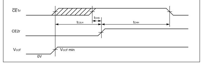
Note: The tc2LH specifies after Vccr reaches specified minimum level.
