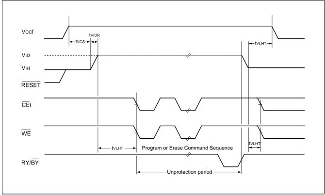
• Acceleration Mode Timing Diagram (Flash)
