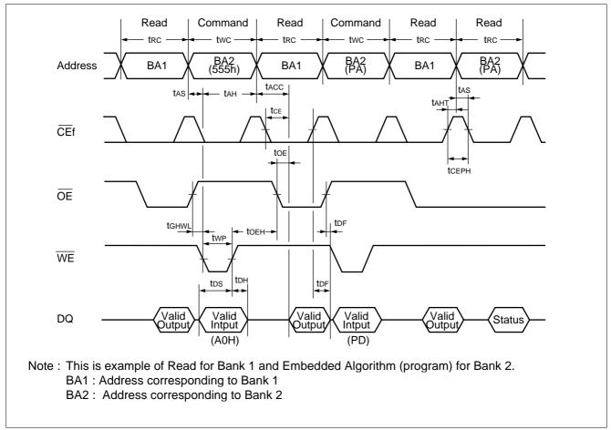
• Back-to-back Read/Write Timing Diagram (Flash)
