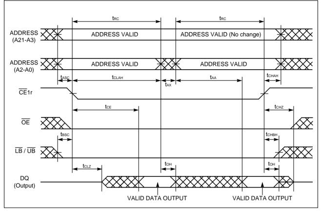
Note: CE2r,  $\overline{PE}$  and  $\overline{WE}$  must be High for entire read cycle. Either or both LB and UB must be Low when both CE1r and OE are Low.
