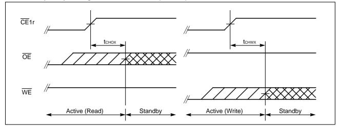
Note: Both t<sub>CHOX</sub> and t<sub>CHWX</sub> define the earliest entry timing for Standby mode. If either of timing is not satisfied, it takes t<sub>RC</sub> (min) period from either last address transition of A0 and A1, or CE1r Low to High transition.
