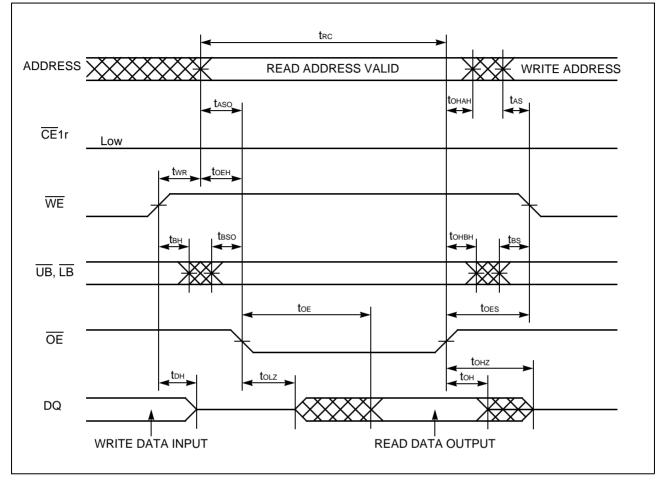
Note:  $\overline{CE}$ 1r can be tied to Low for  $\overline{WE}$  and  $\overline{OE}$  controlled operation. When  $\overline{CE}$ 1r is tied to Low, output is exclusively controlled by  $\overline{OE}$ .
