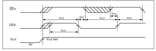
Note: The  $t_{C2HL}$  specifies from CE2r Low to High transition after V<sub>CC</sub>r reaches specified minimum level. CE1r must be brought to High prior to or together with CE2r Low to High transition.
