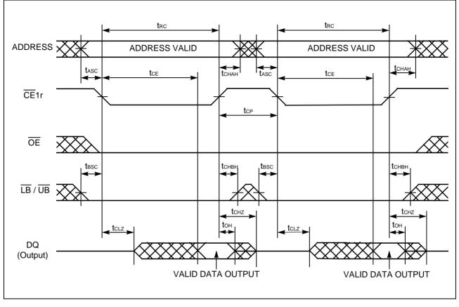
Note: CE2r,  $\overline{PE}$  and  $\overline{WE}$  must be High for entire read cycle. Either or both LB and UB must be Low when both CE1r and  $\overline{OE}$  are Low.
