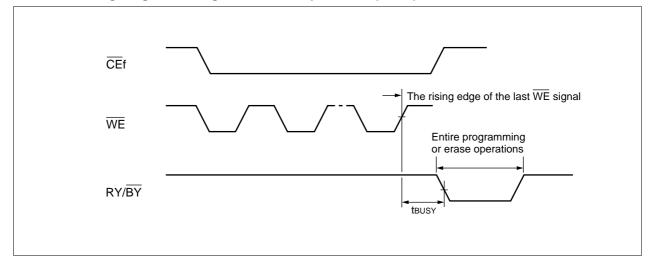
• RESET, RY/BY Timing Diagram (Flash)
