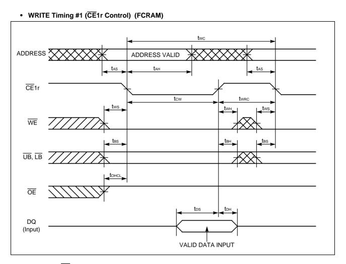
Note: CE2r and  $\overline{PE}$  must be High for write cycle.
