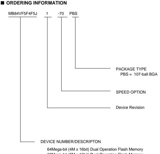
64Mega-bit (4M x 16bit) Dual Operation Flash Memory 32Mega-bit (2M x 16bit) Dual Operation Flash Memory 3.0V-only Read, Program, and Erase
