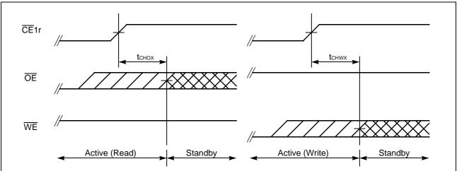
Note: Both tchox and tchwx define the earliest entry timing for Standby mode. If either of timing is not satisfied, it takes trac (min) period from either last address transition of A0 and A1, or CE1r Low to High transition.
