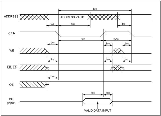
Note: CE2r and  $\overline{\text{PE}}$  must be High for write cycle.
