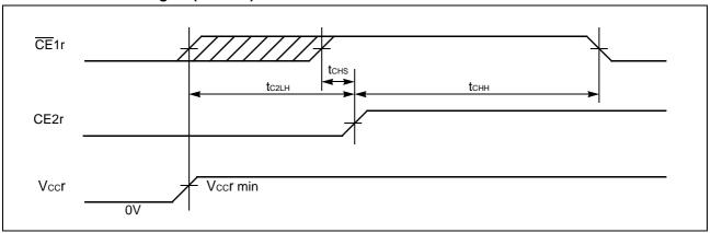
Note: The tc2LH specifies after Vccr reaches specified minimum level.
