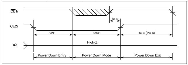
Note: This Power Down mode can be also used for Power-up #2 below except that tchhn can not be used at Power-up timing.
