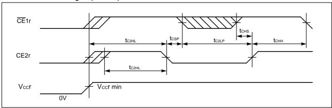
Note: The tc2HL specifies from CE2r Low to High transition after Vccr reaches specified minimum level. CE1r must be brought to High prior to or together with CE2r Low to High transition.
