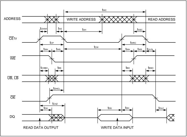
Note: Write address is valid from either  $\overline{CE}1r$  or  $\overline{WE}$  of last falling edge.
