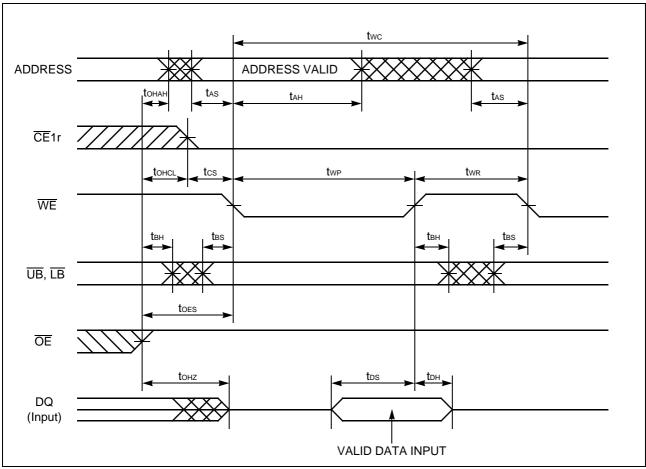
Note: CE2r and  $\overline{PE}$  must be High for write cycle.
