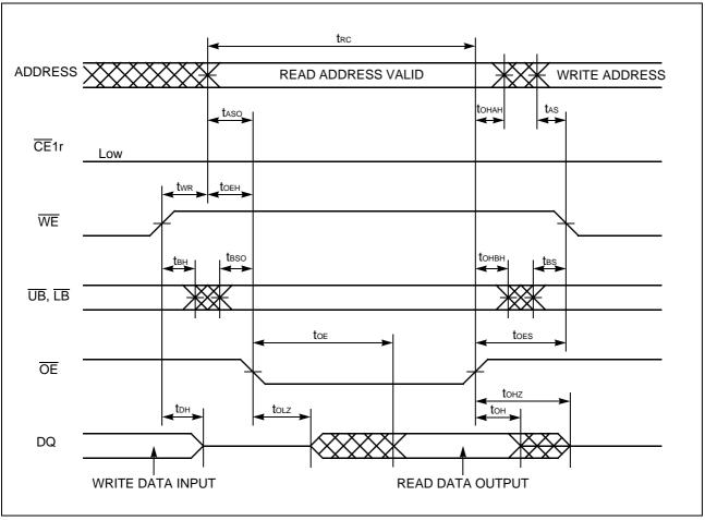
Note:  $\overline{\text{CE}}1\text{r}$  can be tied to Low for  $\overline{\text{WE}}$  and  $\overline{\text{OE}}$  controlled operation. When  $\overline{\text{CE}}1\text{r}$  is tied to Low, output is exclusively controlled by  $\overline{\text{OE}}$ .
