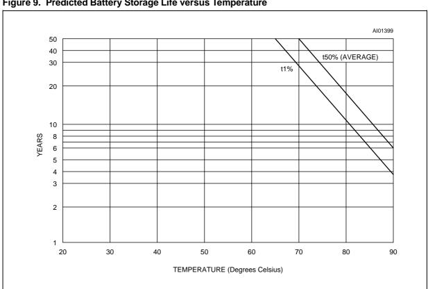
Figure 9. Predicted Battery Storage Life versus Temperature
