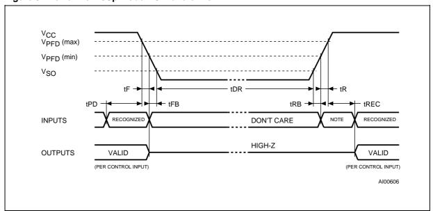
Note: Inputs may or may not be recognized at this time. Caution should be taken to keep  $\overline{E}$  high as  $V_{CC}$  rises past  $V_{PFD}$ (min). Some systems may perform inadvertent write cycles after  $V_{CC}$  rises above  $V_{PFD}$ (min) but before normal system operations begin. Even though a power on reset is being applied to the processor, a reset condition may not occur until after the system clock is running.
