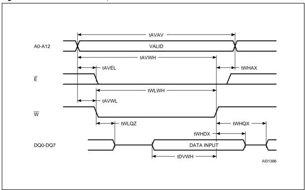
Figure 8. Chip Enable Controlled, Write AC Waveforms
