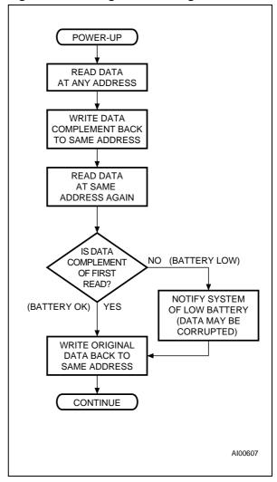
Figure 10. Supply Voltage Protection
