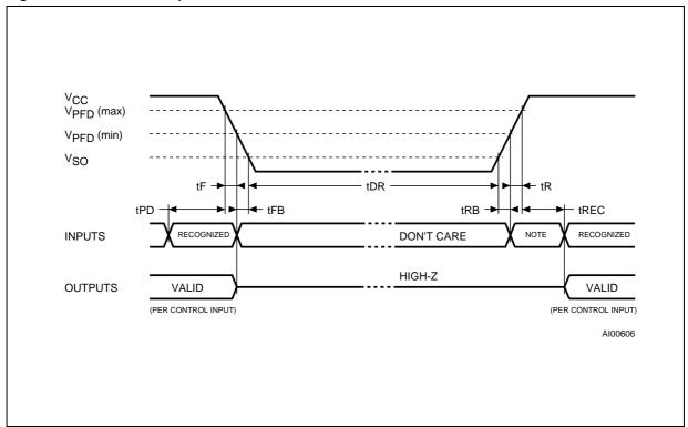
Note: Inputs may or may not be recognized at this time. Caution should be taken to keep  $\overline{E}$  high as  $V_{CC}$  rises past  $V_{PFD}$ (min). Some systems may perform inadvertent write cycles after  $V_{CC}$  rises above  $V_{PFD}$ (min) but before normal system operations begin. Even though a power on reset is being applied to the processor, a reset condition may not occur until after the system clock is running.
