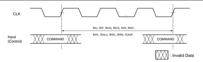
Notes: • These parameters are a limit value of the rising edge of the clock from one command input to the next input. tcksp is the latency value from the rising edge of CKE.
