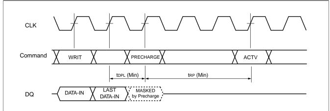
Note: The precharge command (PRE) should only be issued after the topl of final data input is satisfied. PRECHARGE means 'PRE' or 'PALL'.
