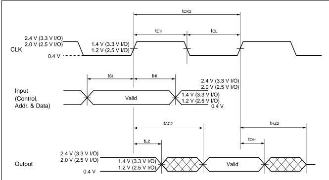
Notes: ● Reference level of input signal is 1.4 V for LVCMOS (3.3 V I/O), 1.2 V for LVCMOS (2.5 V I/O).
