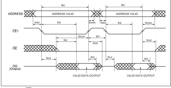
Note : CE2 and  $\overline{\text{WE}}$  must be High for entire read cycle.
