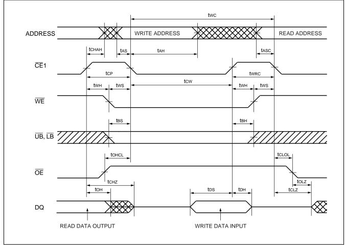
Note : Write address is valid from either  $\overline{CE1}$  or  $\overline{WE}$  of last falling edge.
