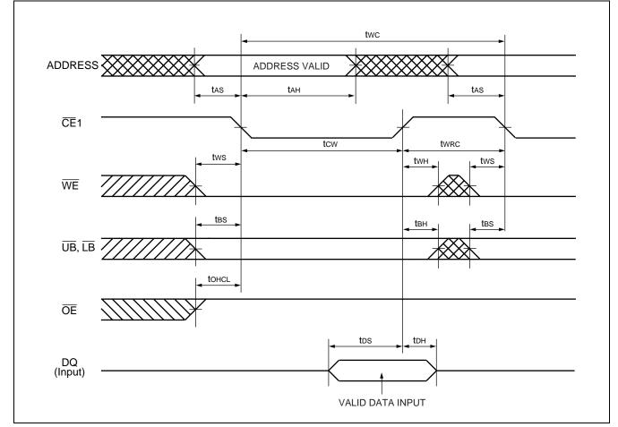
Note : CE2 must be High for write cycle.
