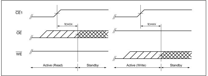
Note : Both t<sub>CHOX</sub> and t<sub>CHWX</sub> define the earliest entry timing for Standby mode. If either of timing is not satisfied, it takes t<sub>RC</sub> (Min.) period from either last address transition of A<sub>0</sub> and A<sub>1</sub>, or  $\overline{CE1}$  Low to High transition.
