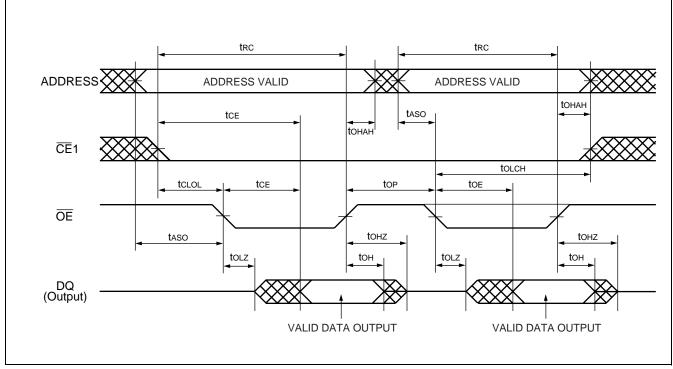
Note : CE2 and  $\overline{\text{WE}}$  must be High for entire read cycle.
