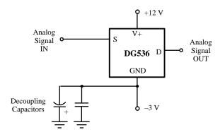
Figure 15. DG536 with Offset Supply
