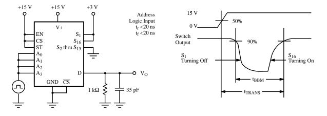
Figure 4. Transition Time and Break-Before-Make Interval
