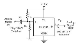
Figure 14. Simple Bias Circuit
