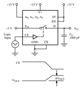
$\Delta V_{OUT}$  is the measured voltage error due to charge injection. The charge injection in Coulombs is Q = C<sub>L</sub> x  $\Delta V_{OUT}$
