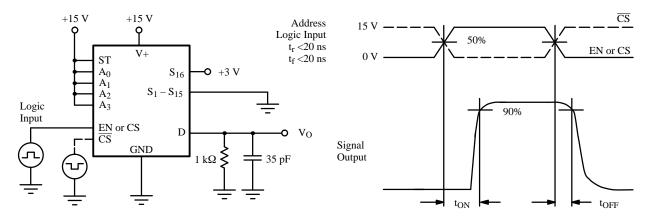
**Figure 2.** EN, CS,  $\overline{CS}$ , Turn On/Off Time
