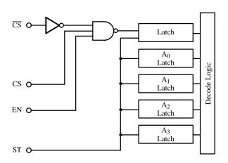
Figure 11. CS, CS, EN, ST Control Logic
