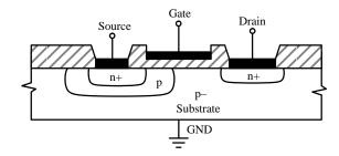
Figure 13. Cross-Section of a Single DMOS Switch
