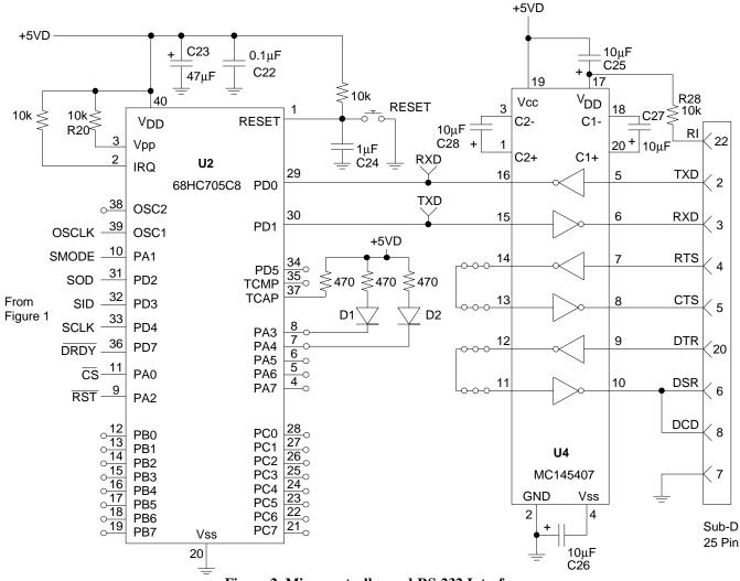
Figure 2. Microcontroller and RS-232 Interface
