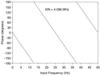
Figure 12. Filter Phase Response.
