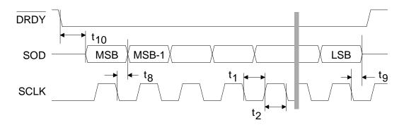
**SOD** Read Timing with CS = 0 (Not to Scale)
