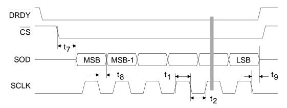
**SOD Read Timing (Not to Scale)**
