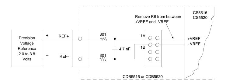
Figure 6. Using Off-board Voltage Reference
