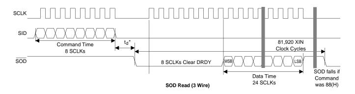
Figure 4. Command and Data Word Timing
