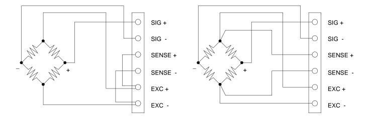
Figure 4. 4-Wire Bridge Connections
