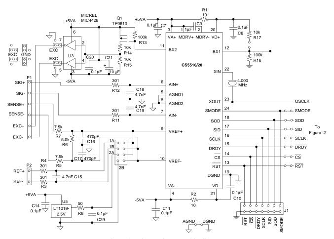
Figure 1. Bridge Driver and A/D Converter
