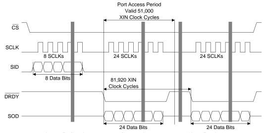
Figure 5. Continuous Read Conversion Data Mode (4 or 5 Wire)
