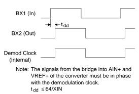
Figure 8. External Excitation Clock Phasing
