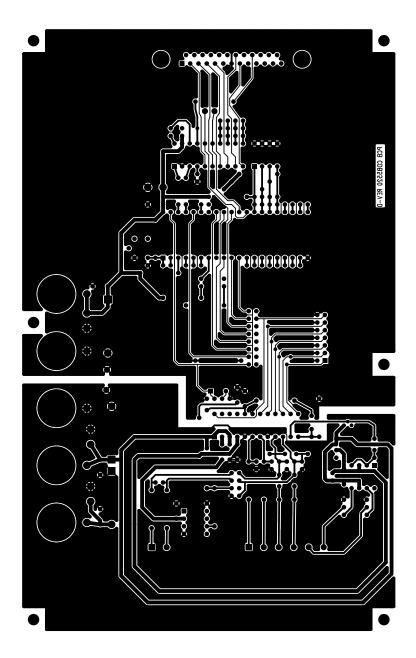
Figure 10. CDB5520 Solder Side Trace Layer
