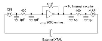
Figure 10. On-Chip Gate Oscillator Model
