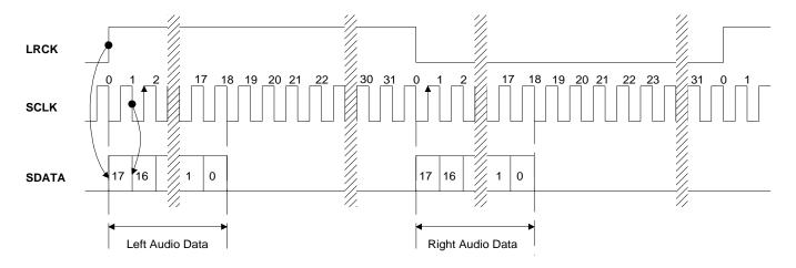
Figure 2. Data Output Timing - CS5330A
