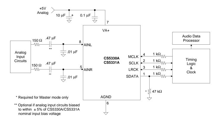
Figure 1. Typical Connection Diagram
