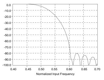
Figure 8. CS5330A/31A Digital Filter Transition Band
