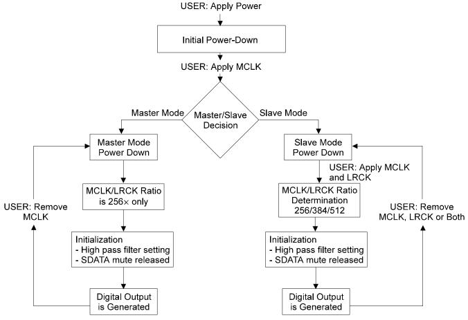
Figure 4. CS5330A/31A Initialization and Power-Down Sequence
