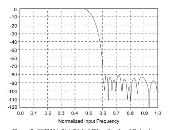
Figure 5. CS5330A/31A Digital Filter Stopband Rejection
