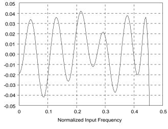
Figure 7. CS5330A/31A Digital Filter Passband Ripple
