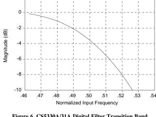
Figure 6. CS5330A/31A Digital Filter Transition Band
