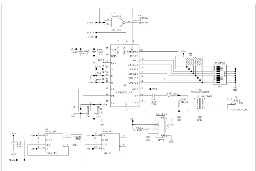
Figure 4. CS8402A Digital Audio Transmitter Connections
