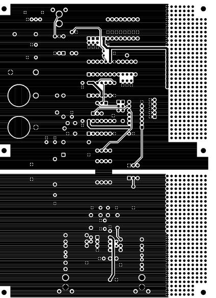
Figure 9. CDB5330A/31A Solder Side (bottom)
