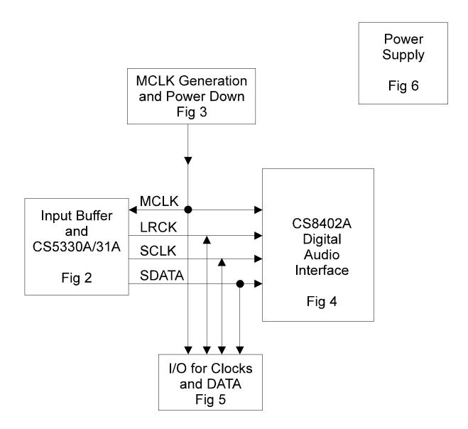
Figure 1. System Block Diagram and Signal Flow
