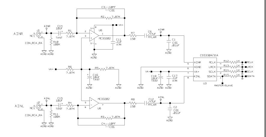
Figure 2. CS5330A/31A and Connections
