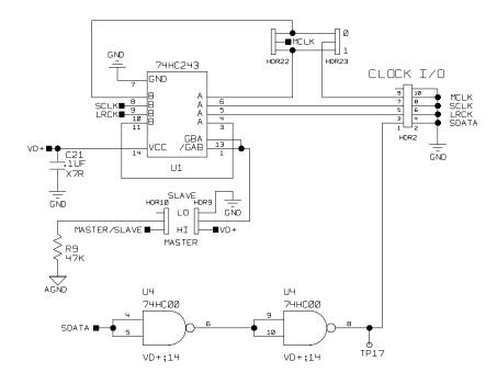
Figure 5. I/O Interface for Clocks and Data
