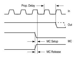
Modulus setup time MC to out is the MC setup or MC release plus the prop delay.
