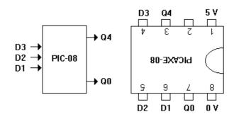
Both the PICAXE-18 and PICAXE-08 can hold programs up to 128 bytes in length, corresponding to about 40 separate commands in BASIC.
