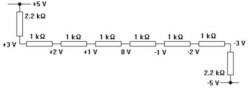
2 Now connect the seven reference voltages to the inputs of a 4051 multiplexer, as shown below. Pin 7 of the multiplexer i.c. will need to be connected to -5 V, to allow negative signals through to the output. Assemble the rest of the circuit.
