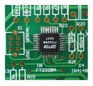
**NOTE:** the two adjacent pins 13 & 14, (3<sup>rd</sup> & 4<sup>th</sup> pins from the top left) are connected together. If you see a solder bridge between these pins is OK and not a mistake. Pins 3, 13, 14, & 26 are connected to Vcc.
