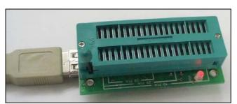
Fitting into the Box. Our original idea was to screw the PCB into the box provided. However, as you can see the heads of the screws will hit the ZIF socket. So what we have done is made the pcb slightly over-width so some filing will be needed to tight fit the pcb into the box so no screws are required.
