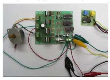
We used the debounced Counter Module of our Kit 1 to test Kit 158. You can get the schematic for it here <a href="http://www.kitsrus.com/pdf/k1.pdf">http://www.kitsrus.com/pdf/k1.pdf</a>
