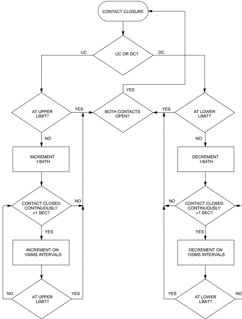
CONTACT OPEN AND CONTACT CLOSURE TIMING IS one second  $\pm$  15%
