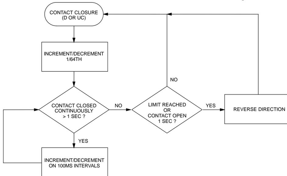
CONTACT OPEN AND CONTACT CLOSURE TIMING IS one second  $\pm$  15%
