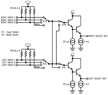
FIGURE 2. Input and Mode Select Circuitry
