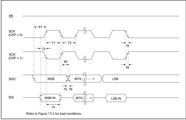
FIGURE 17-10: SPI SLAVE MODE TIMING (CKE = 0)
