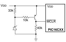
Note 1: This circuit will activate reset when VDD goes below (Vz + 0.7V) where Vz = Zener voltage.
