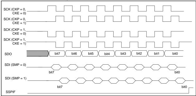
FIGURE 11-6: SPI MODE TIMING (SLAVE MODE WITH CKE = 0)
