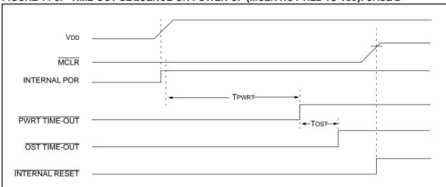
FIGURE 14-10: TIME-OUT SEQUENCE ON POWER-UP (MCLR TIED TO VDD)
