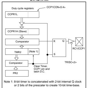
A PWM output (Figure 10-5) has a time-base (period) and a time that the output stays high (duty cycle). The frequency of the PWM is the inverse of the period (1/period).
