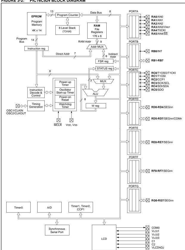
FIGURE 3-2: PIC16C924 BLOCK DIAGRAM
