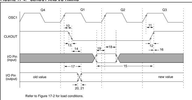
FIGURE 17-4: CLKOUT AND I/O TIMING
