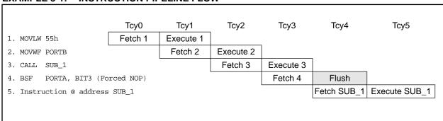
All instructions are single cycle, except for any program branches. These take two cycles since the fetch instruction is "flushed" from the pipeline while the new instruction is being fetched and then executed.
