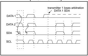
Masters that also incorporate the slave function, and have lost arbitration must immediately switch over to slave-receiver mode. This is because the winning master-transmitter may be addressing it.
