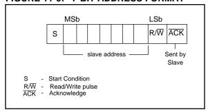
FIGURE 11-10: I<sup>2</sup>C 10-BIT ADDRESS FORMAT
