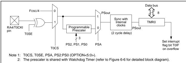
FIGURE 6-2: TIMER0 TIMING: INTERNAL CLOCK/NO PRESCALE
