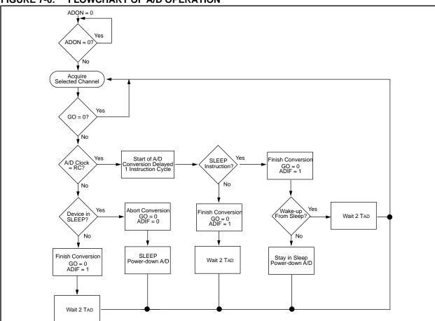
FIGURE 7-6: FLOWCHART OF A/D OPERATION
