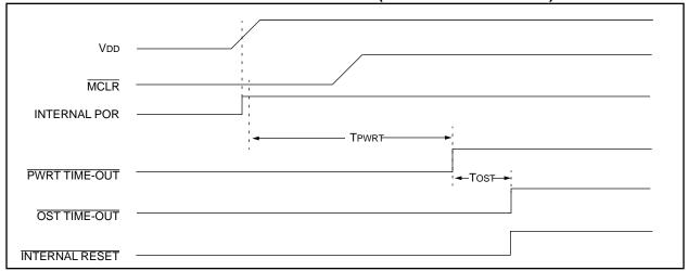
FIGURE 8-10: TIME-OUT SEQUENCE ON POWER-UP (MCLR NOT TIED TO VDD): CASE 2
