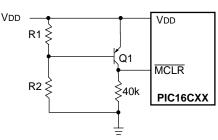
Note 1: This brown-out circuit is less expensive, albeit less accurate. Transistor Q1 turns off when VDD is below a certain level such that:
