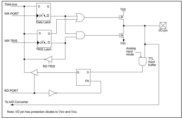
FIGURE 5-2: BLOCK DIAGRAM OF RA4/T0CKI PIN
