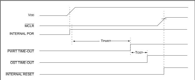
FIGURE 8-11: TIME-OUT SEQUENCE ON POWER-UP (MCLR TIED TO VDD)
