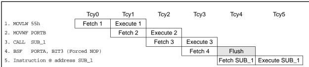
All instructions are single cycle, except for any program branches. These take two cycles since the fetch instruction is "flushed" from the pipeline while the new instruction is being fetched and then executed.
