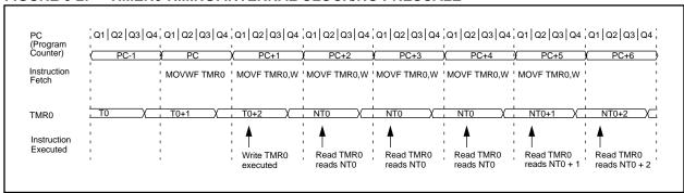
FIGURE 6-3: TIMERO TIMING: INTERNAL CLOCK/PRESCALE 1:2
