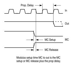
Figure 3. Typical Output Waveform
