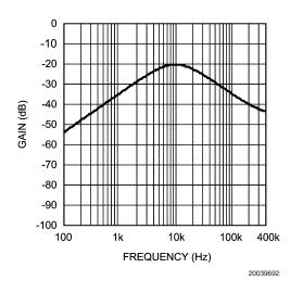
FIGURE 11. Bandpass Filter Frequency Response
