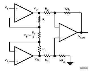
FIGURE 1. Instrumentation Amplifier
