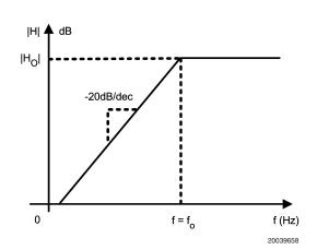
FIGURE 6. Highpass Filter Transfer Function
