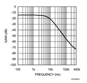
FIGURE 10. Lowpass Filter Frequency Response
