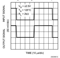
Non-Inverting Large Signal Pulse Response
