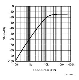
FIGURE 12. Highpass Filter Frequency Response
