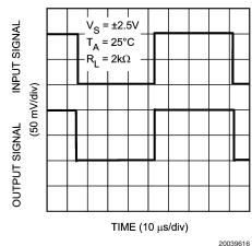
Non-Inverting Small Signal Pulse Response
