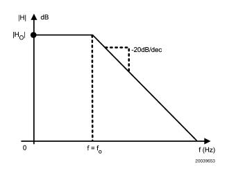
FIGURE 4. Lowpass Filter Transfer Function
