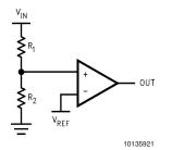
**FIGURE 4. Threshold Detector**
