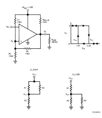
FIGURE 1. Inverting Comparator with Hysteresis
