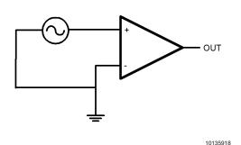
FIGURE 3. Zero-Crossing Detector
