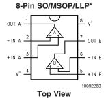
Note: LLP-8 exposed DAP can be electrically connected to ground for improved thermal performance.
