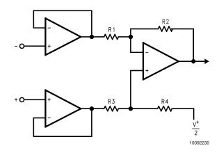
FIGURE 6. Three-op-amp Instrumentation Amplifier
