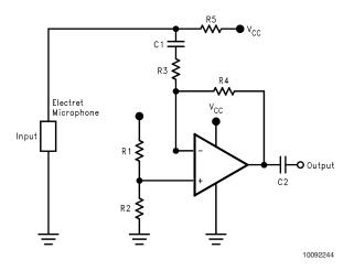
FIGURE 11. A Battery Powered Microphone Preamplifier
