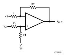
$$\begin{split} &V_{OUT} = \left(\frac{R1 + R2}{R3 + R4}\right)\frac{R4}{R1}V_2 - \frac{R2}{R1}V_1 + \left(\frac{R1 + R2}{R3 + R4}\right)\frac{R3}{R1} \cdot \frac{V^4}{2} \\ &\text{for R1} = R3 \text{ and } R2 = R4 \\ &V_{OUT} = \frac{R2}{R1}\left(V_2 - V_1\right) + \frac{V^4}{2} \end{split}$$
