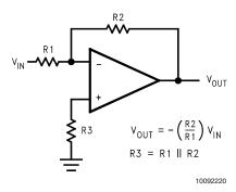
FIGURE 4. Cancelling the Error Caused by Input Bias
