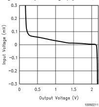
Input Offset Voltage vs. Input Common-Mode Voltage Range  $V_S = 2.2V$
