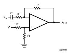
$$V_{OUT} = -\frac{R2}{R1}V_{IN}$$
