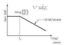
FIGURE 10. Frequency Response of Simple Low-pass
