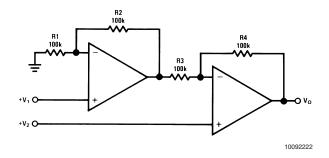
$V_0 = \left(1 + \frac{R4}{R3}\right) (V_2 - V_1)$ , where R1 = R4 and R2 = R3 As shown:  $V_0 = 2(V_2 - V_1)$
