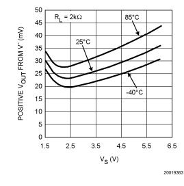
**Output Negative Swing vs. Supply Voltage**
