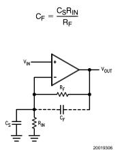
$C_S$  consists of the amplifier's input capacitance plus any stray capacitance from the circuit board and socket.  $C_F$  compensates for the pole caused by  $C_S$  and the feedback resistors.
