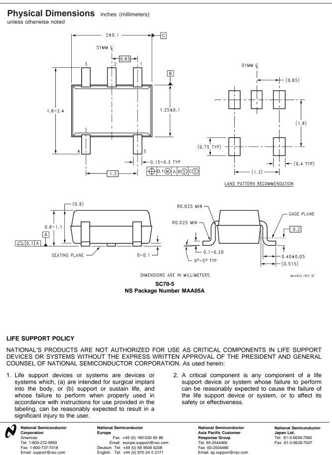
LMV301 Low Input Bias Current, 1.8V Op Amp w/ Rail-to-Rail Output
