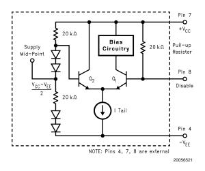
FIGURE 4. Enable/Disable Operation
