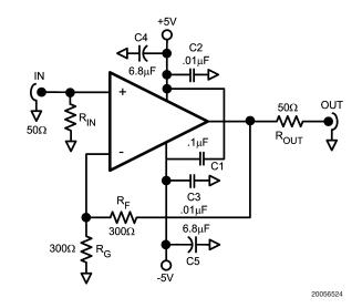
FIGURE 5. Typical Application with Suggested Supply Bypassing
