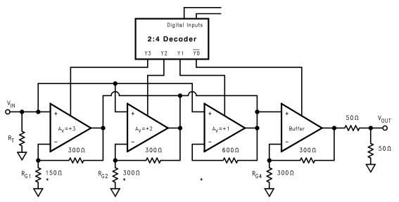
\*NOTE: Selectable gains can be changed by using different  $R_{\mbox{\scriptsize g}}$  resistors.
