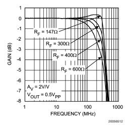
FIGURE 1. Frequency Response vs. R<sub>F</sub>
