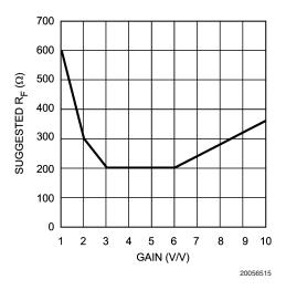
FIGURE 2. R<sub>F</sub> vs. Non-Inverting Gain
