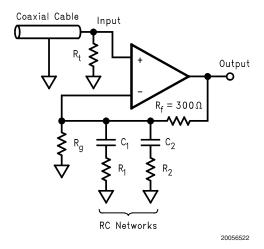
FIGURE 8. Equalizer Circuit Schematic
