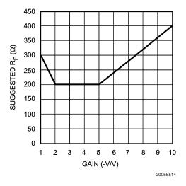
FIGURE 3. R<sub>F</sub> vs. Inverting Gain
