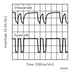
FIGURE 9. Digital Signal without and with Equalization
