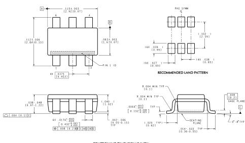
CONTROLLING DIMENSION IS INCH VALUES IN [ ] ARE MILLIMETERS
