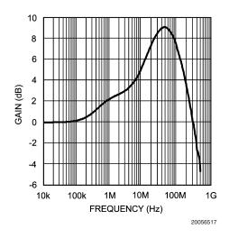
FIGURE 11. Equalizer Frequency Response
