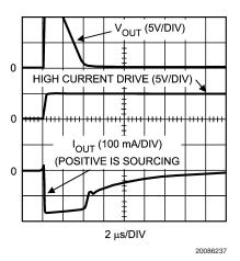
FIGURE 3. Expanded View of Figure 2 Waveforms showing LMH6640 Current Sinking 1/2 Cycle
