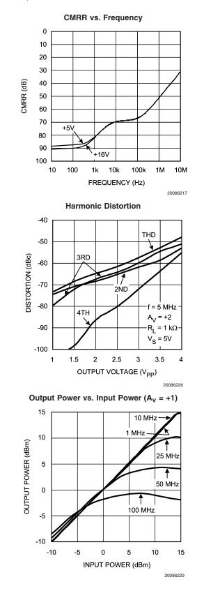
**Typical Performance Characteristics** At  $T_J = 25^{\circ}C$ ,  $V^+ = 16$  V,  $V^- = 0V$ ,  $R_F = 330\Omega$  for  $A_V = +2$ ,  $R_F = 1 \ k\Omega$  for  $A_V = -1$ .  $R_L$  tied to  $V^+/2$ . Unless otherwise specified. (Continued)
